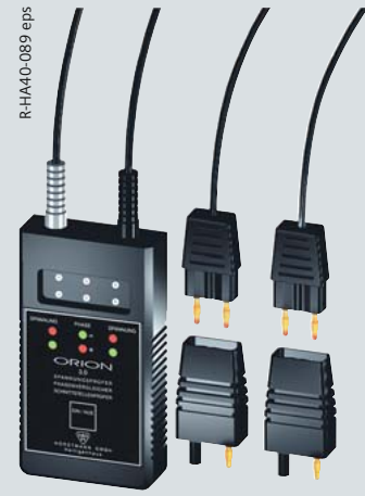
Phase comparison test unit make Horstmann, type ORION 3.0 as combined test unit for: – Phase comparison – Interface testing at the switchgear – Voltage detection for LRM systems – Integrated self-test – Indication via LED and acoustic alarm
